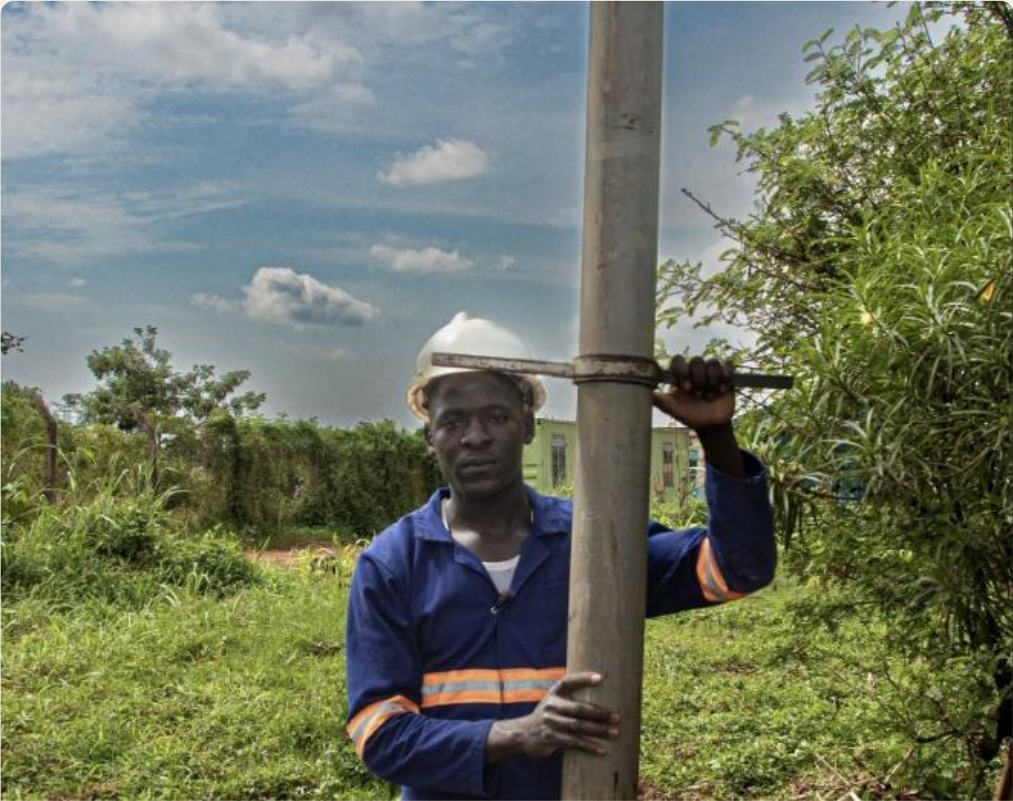
Gulper: a hand pump lifting sludge into drums, about 3 litres per stroke
